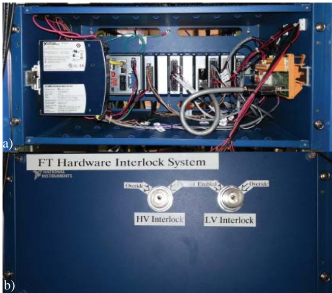
FIG. 2. FT cRIO chassis. a) Front panel removed, showing interior, b) front panel, with keyed switches.
